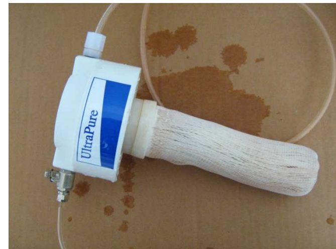
The DUC410 cartridge after rinsing with clean water
