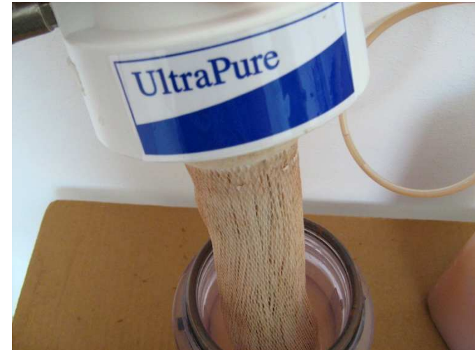
Debris trapped in the DUC410 cartridge
